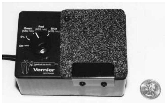
Figure 1. Colorimeter sensor unit from Vernier Software [8].
