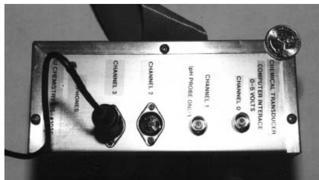
Figure 3. Routing box for analog transducers.
